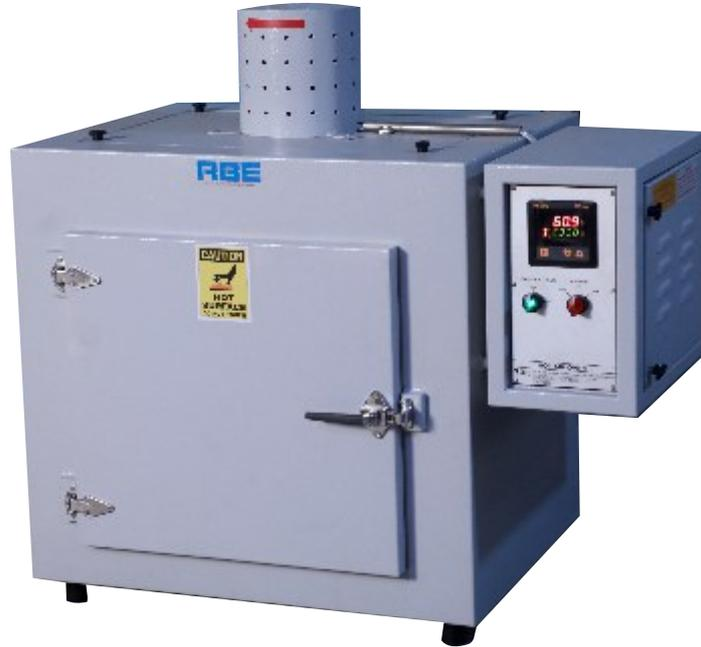
Laboratory OVEN is used in laboratory applications such as Drying and Curing of fabric and yarn samples and also used in tests like perspiration tests, Double walled chamber with inner wall of SS, blower for uniform heat distribution all over the chamber, SS Perforated trays for keeping samples.
