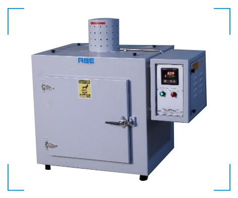
Laboratory OVEN is used in laboratory applications such as Drying and Curing of fabric and yarn samples and also used in tests like perspiration tests, Double walled chamber with inner wall of SS, blower for uniform heat distribution all over the chamber, SS Perforated trays for keeping samples.
