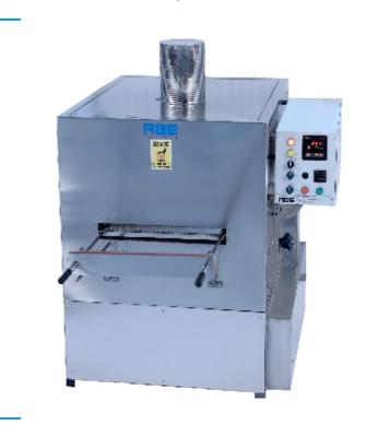
A compact table top machine suitable to do the Drying / Curing trials in Laboratory for small samples attaching on pin frame with adjustable position of the pins on the frame for different size of samples. Automatic ejection of the pin frame from the hot zone on completion of the set dwell time. Machine is provided with blowers for Hot air recirculation
