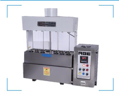
Machine is used for dyeing of fabric, yarn & loose stock samples. The rocking bars, apart from up-down motion, rotate at 70 RPM. Direction reversal of rocking bars rotation after every 3 mins. This ensures proper contact between substrate & liquor due to constant agitation in liquor.
