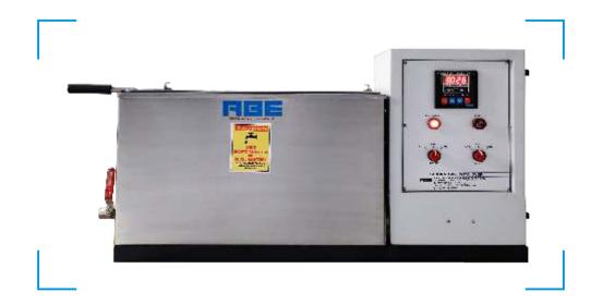
Rota Dyer is used for shade matching and for testing of various types of dyes up to dyeing temperature of 95°C.
