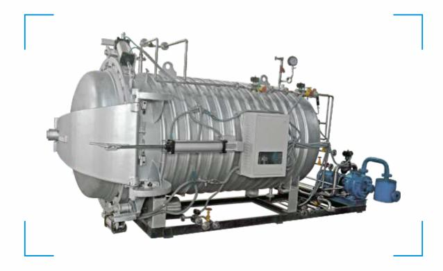
A production machine for spinners to achieve twist setting, yarn conditioning, bulking, and top to tow conversion of acrylic yarn. Yarn is subjected to vacuum and pressure to the required levels in a sealed autoclave. Machine equiped with Fully computerized control system with necessary logical Interlock and alarms. Improves efficiency in weaving winding and dyeing due to conditioning of yarn & Stabilizes moisture content in the yarn.
