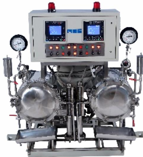
A Laboratory model Yarn setting machine with multiple chamber to carry out the lab trials in yarn for twist setting, conditioning bulking etc. different kind of trials with different parameters can be carry out simultaneously in each chambers .
