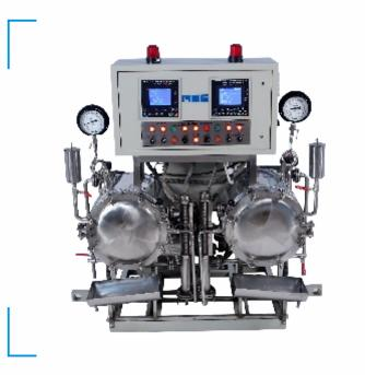
A Laboratory model Yarn setting machine with multiple chamber to carry out the lab trials in yarn for twist setting, conditioning bulking etc. different kind of trials with different parameters can be carry out simultaneously in each chambers.
